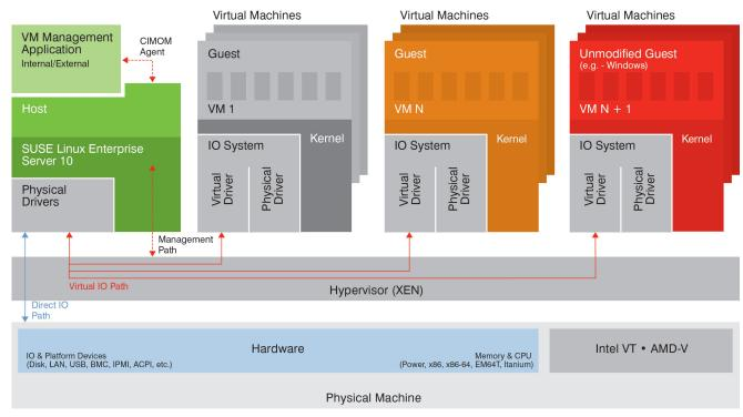
Figure 1. The Xen architecture enables virtualized operating systems to talk directly to hardware, with minimal impact on performance.
